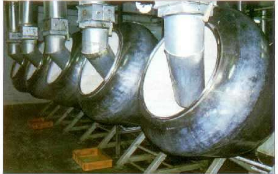
A battery of coating pans. Photo courtesy of Gansons Ltd.
